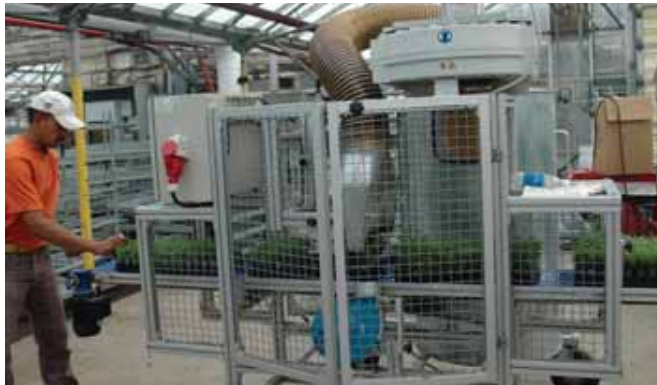
Figure 5. Mechanization of liner shearing.
