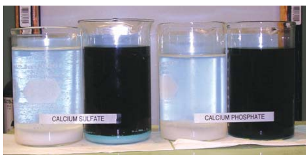
Figure 1. Incompatible formulations: These four beakers contain a concentrate of 15-0-15 Dark Weather fertilizer. The clear beakers contain a No-Dye formula. Magnesium sulfate (Epson salts) was added to the two beakers on the left. The precipitate that formed is calcium sulfate. Potassium phosphate was added to the two beakers on the right and the precipitate that formed is calcium phosphate.
