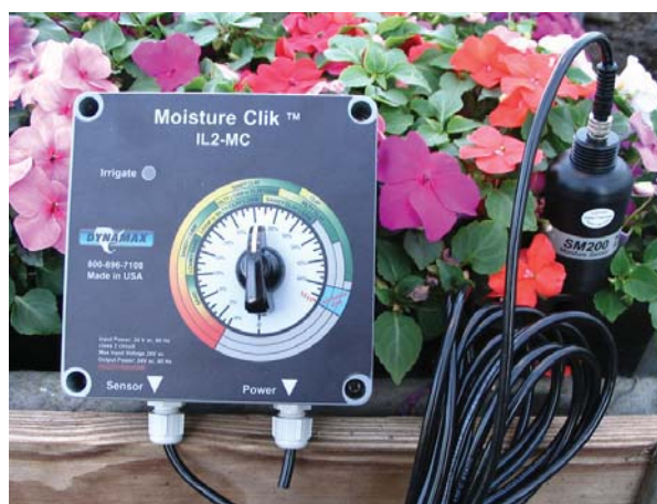
Figure 4. The Moisture Klik™ irrigation controller from Dynamax uses an SM200 moisture sensor. When the substrate water content drops below the set point, the irrigation is turned on until the water content is raised above the set point.
