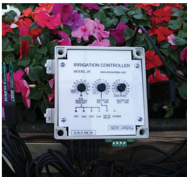
Figure 3. The single-zone irrigation controller from Brower Electronics Labs uses one to four ECH 2 O-5 probes from Decagon to measure the substrate water content. As the water content drops below the set point, irrigation can automatically be turned on.
