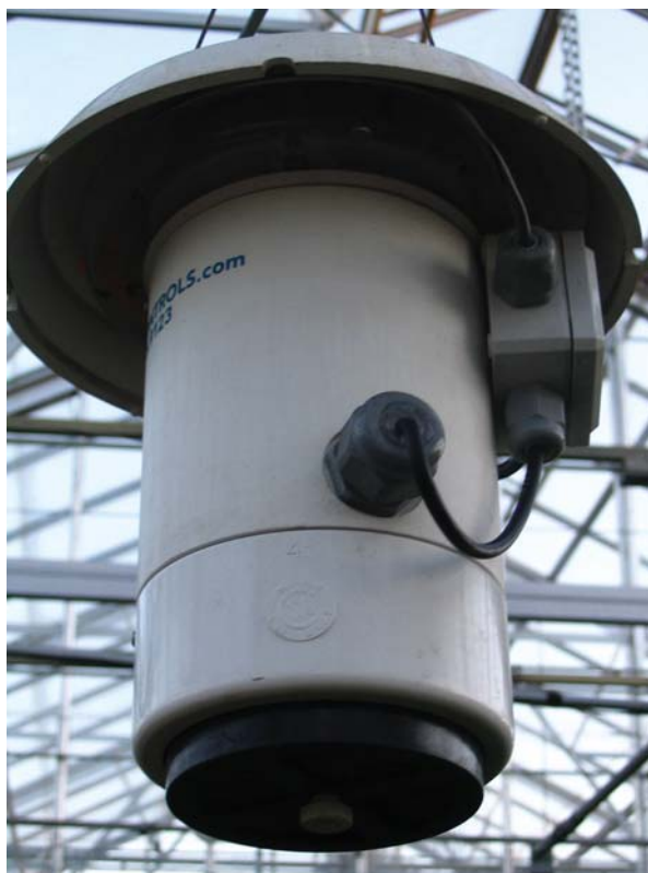
Figure 2. Temperature and humidity sensors should be inside an enclosure that keeps the sensors shaded. The enclosure has a filter and fan to provide adequate air flow past the sensor. Make sure to clean the filter and check the fan regularly. A broken fan may cause temperature readings to be too high.
