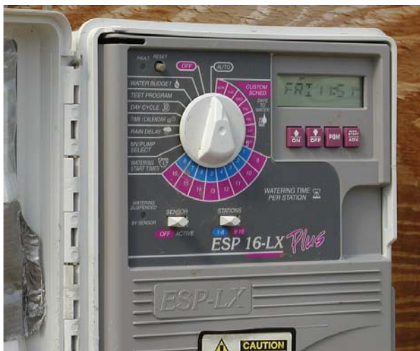
Figure 1. Irrigation timers are the simplest way to automatically turn irrigation on and off. Unfortunately, they cannot automatically adjust the watering schedule according to the changing water needs of the plants.
