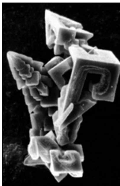
Figure 3. Chlorothalonil crystal viewed with SEM at X 10,000.
